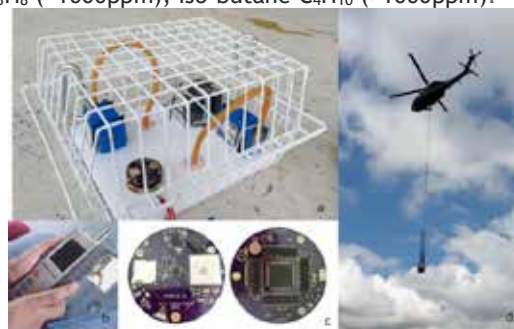
Figure 1.a) Measurement instruments disposition: Particle counter OPC-N3, nanofilter experiments and GilAir 3 air pump disposition and Simple unit, b) Laser Particle counter, c) Simple CO&DH subsystem, d) Aircraft external load configuration.
