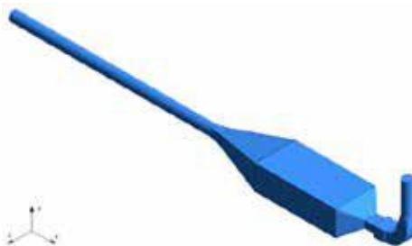
Figure 2. Schematic drawing of the modified geometry: extended straight inlet (Case B)
