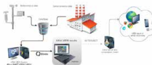
Figure 1: Representative scheme of the ARIA View system
