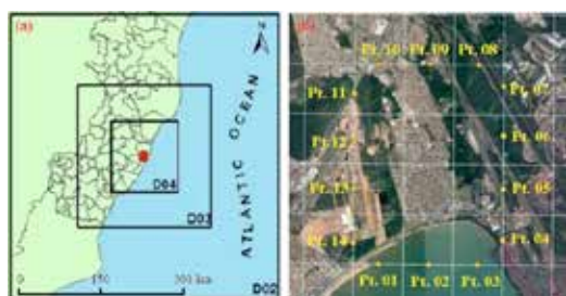
Figure 2. (a) Mesoscale model domains and (b) details of the domain D04 and the points that delimit the neighborhood.
