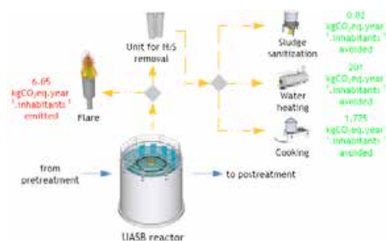
Figure 1. Schematic representation of the proposed different biogas usages in small-scale STPs.
