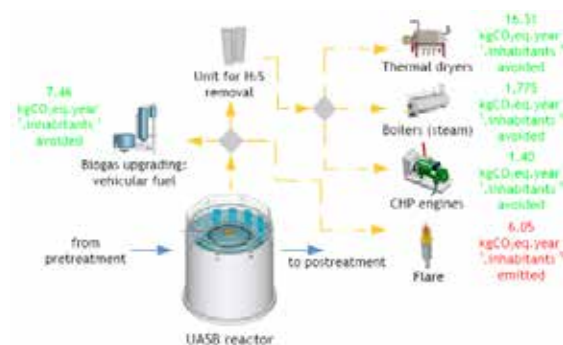
Figure 3. Schematic representation of the proposed different biogas usages in large-scale STPs.
