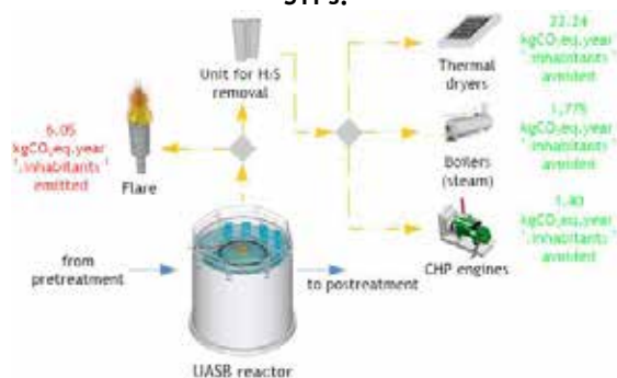
Figure 2. Schematic representation of the proposed different biogas usages in medium-scale STPs.
