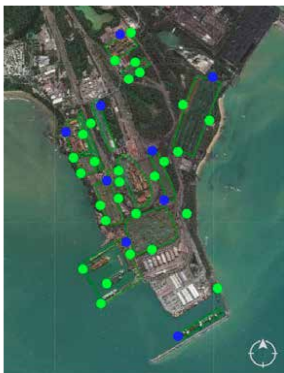
Figure 1. RAMP: Automatic network for the monitoring fugitive PM emissions installed in an Industrial Complex (Vitória, ES, Brazil). Circles indicate profiling towers. Blue circles indicate stations equipped also with wind sensors.
